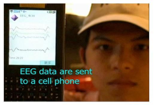
**Dry electrode wireless EEG cap:** Tzyy-Ping Jung in collaboration with researchers in Taiwan has developed EEG systems which can monitor brainwaves remotely, and without the tiresome application of gel electrodes.
